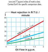
Comparable heat rejection rates based on
