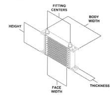
**TEMP-A-CURE oil coolers** are designed to suit any application. The chart below will assist you in choosing the correct model for your needs.
