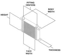
Earl's curved coolers are constructed with the same high grade aluminum and the same internal design as our standard 2" coolers, but have a curved design to fit neatly between the front forks of a motorcycle for maximum heat dissipation. The curved design allows for full wheel travel no matter where it is mounted on the forks. These coolers are only 1-1/4" thick and are available in two widths, three different heights and male -6 or -8 inlet and outlet fittings.
