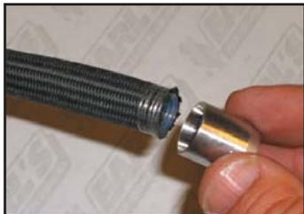
4. Insert crimp collar onto UltraFlex hose. Do not remove thin tape as adhesive from tape might unravel Kevlar braid.
