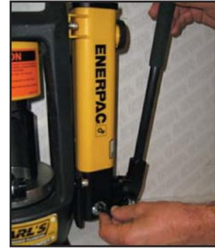
12. While holding hose and fitting into position, begin pumping hand pump until die ring contacts crimper base plate. Release pressure by turning triangular knob on valve.
