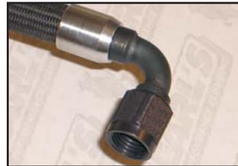
6. Insert UltraFlex fitting nipple into collar and hose assembly as shown.
