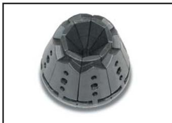
8. Verify correct size crimp die. When inserting die into crimper insure that the bottom of die (shown) mates correctly with die bowl and diamond shaped features in die bowl.
