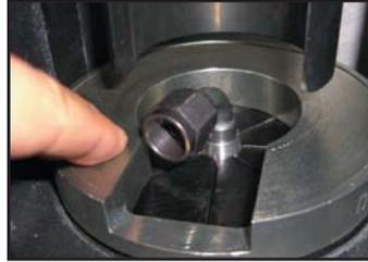
11. Insert and position the hose and fitting assembly into crimp from below. Verify that crimp collar seats correctly in crimp die.
