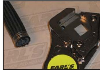
3. Cut hose square or perpendicular to centerline of hose. No loose or fraying Kevlar braids are to be present.
