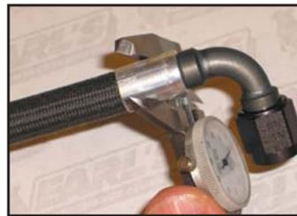
14. Measure crimp diameter to ensure proper crimp diameter has been achieved. Refer to crimp chart dimension chart.
