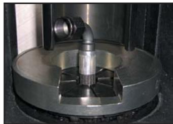
13. Remove hose and fitting assembly through bottom of die ring and inspect crimp on hose assembly.
