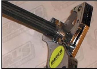
2. Use the Earl's UltraFlex Hand Hose Cutter to cut hose. Use a sharp blade as to not crush the Teflon® hose during the cutting process.
