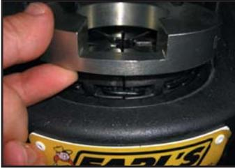
10. Gently push down onto crimp die to insert and center die ring on top of crimp die below pusher. Verify that bottom of crimp die is seated correctly in die bowl. Prepare to install pusher onto crimper.
